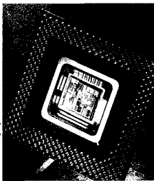
FIGURE 1.2 A Pentium ® chip with 3.3 million transistors. Such microprocessors are at the heart of today's personal computers. (Courtesy of Intel Corporation.)
