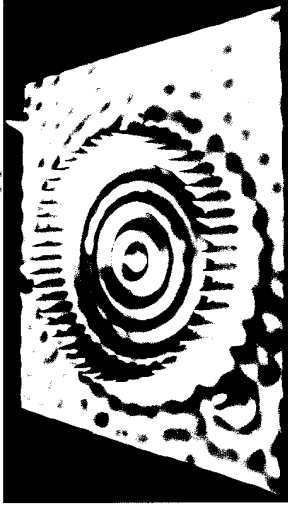
FIGURE 1.3 A scanning tunneling microscope (STM) image that shows the wavelike nature of electrons confined within a “quantum corral,” 14 nanometers in diameter, made up of 48 individually positioned iron atoms on a copper surface. Devices formed by precise positioning of atoms or molecules may one day play an important role in ultrahigh-performance computer chips. (Courtesy of IBM Research.)
