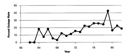
The contributions to forced outages for calendar year 1982 are analyzed in Table 4 below. These data show that cyclone failures were the principal cause of the unit's degraded performance.
