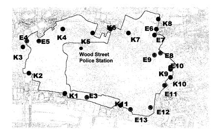
At each entry point the highway layout was amended to force vehicles to slow down and allow Police officers to interview occupants if necessary. At each of these locations a series of high performance cameras were deployed along with specialist lighting. The cameras systems allowed a clear view to be obtained of each vehicle and its occupants.
