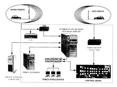
The cameras are linked to the Force headquarters and control room via a dedicated resilient fibre optic network to minimise any downtime or possibility of sabotage. The information and images transmitted by the cameras are used to read the licence plate using an automated process. The index number is then matched on the Police National Computer. Should a match occur, specific information is delivered to the police control room. This may include:
