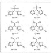
Figure 1: Chemical structures of isomers of DDT, DDE, and DDD
