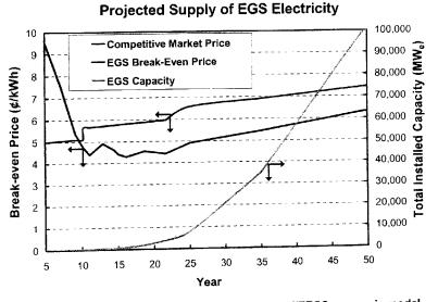
Figure 4. Estimated supply curve for EGS based on the MITEGS economic model. (from *The Future of Geothermal Energy*, MIT Report, Cambridge, MA (2006)
