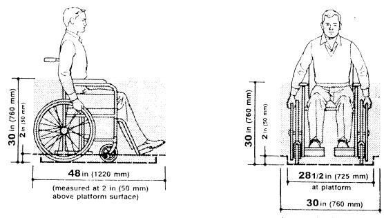
(measured at 2 in (50 mm) above the platform surface)
