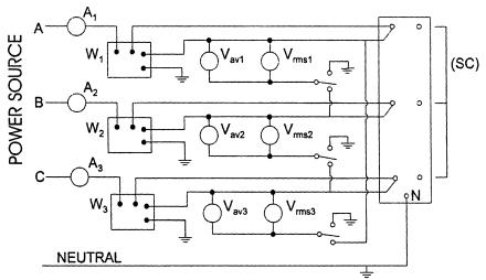
Figure 4.3 Three-Phase Test Set Without Instrument Transformers
