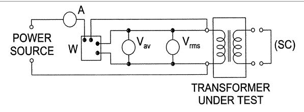
Figure 4.1 Single-Phase Test Set Without Instrument Transformers
