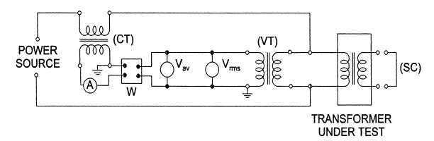
Figure 4.2 Single-Phase Test Set With Instrument Transformers
