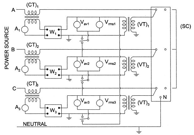
Figure 4.4 Three-Phase Test Set with Instrument Transformers
