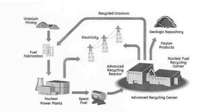
Figure 2: GEH Advanced Recycling Center to close the fuel cycle in the future.
