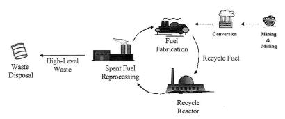
Figure 2. Closed nuclear fuel cycle (or reprocessing/recycling)
